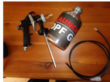
2. Unscrew the trigger section from the fluid container. When using Launch DPF Gun Fluid, mix the fluid with water at 1 part DPF Fluid to 2 parts water for normal application, or 1 part DPF Fluid to 1 part water for heavily contaminated DPF's.
