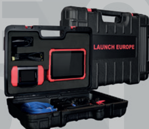
BENZ 38, BENZ 14, BMW 20, OBD I Adapter Box, 16-pol OBD-Bluetooth Adapter, Double Clamp Power Line, Cigarette Lighter Line, Extension Line, PIN Envelope
